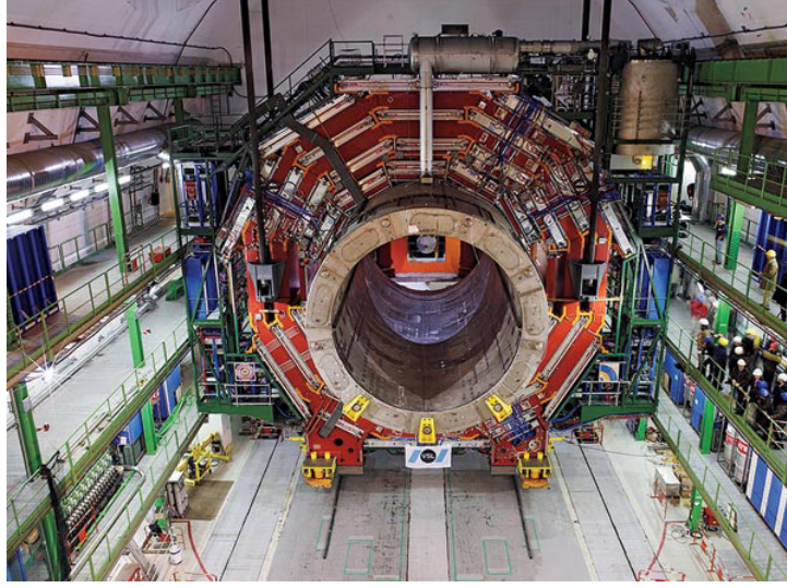
Figure 2.5: Bore of the CMS solenoid being inserted within the muon chambers interspersed with the steel yokes at the surface.
